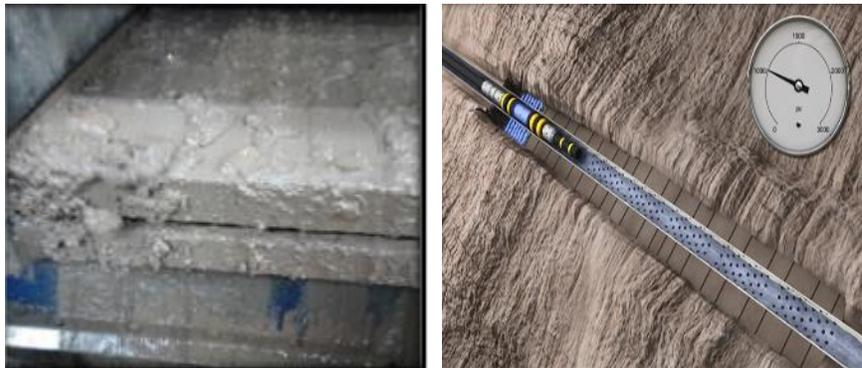
4. Once washing is completed, engage inline spear (LOCK® plug) and pull to retrieve casing. Tensile rating up to 300MT
