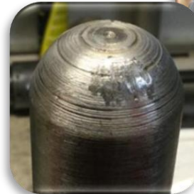
Failure to drift – hang up at tubing hanger
