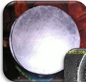
Drift impression of upper velocity string (ER Packer)
