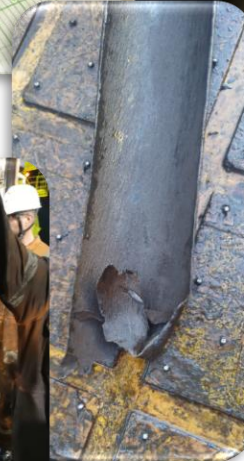
Corroded tubing fish – cut from spear on rig floor
