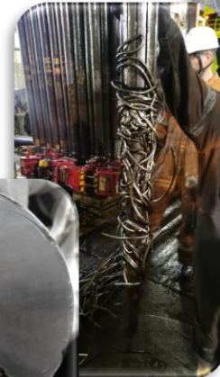
Fished control line (tubing corroded)
