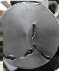
LIB impression following drift failure
