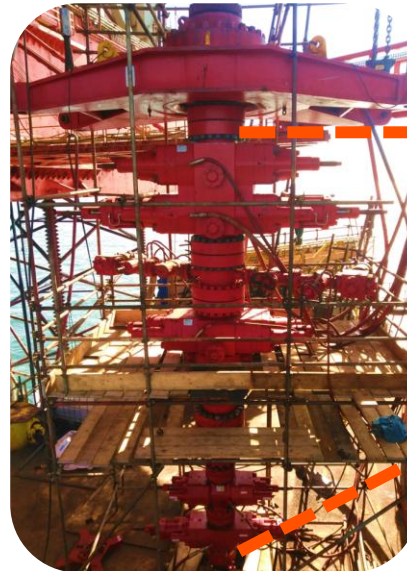
Bespoke BOP: (7 1/16" rams integrated into rig BOP stack)
