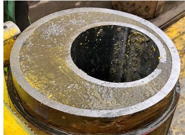
Inspection: Fully cemented cross-section
