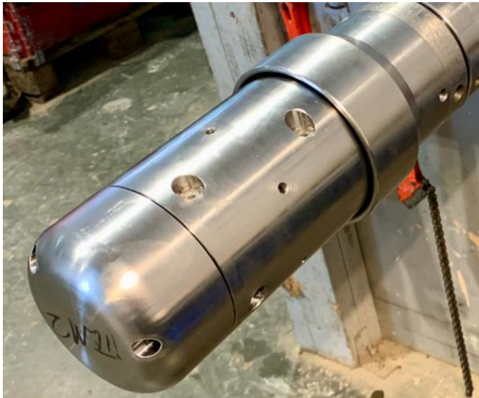
Jet Propulsion Rotating Washing and Cement Head
