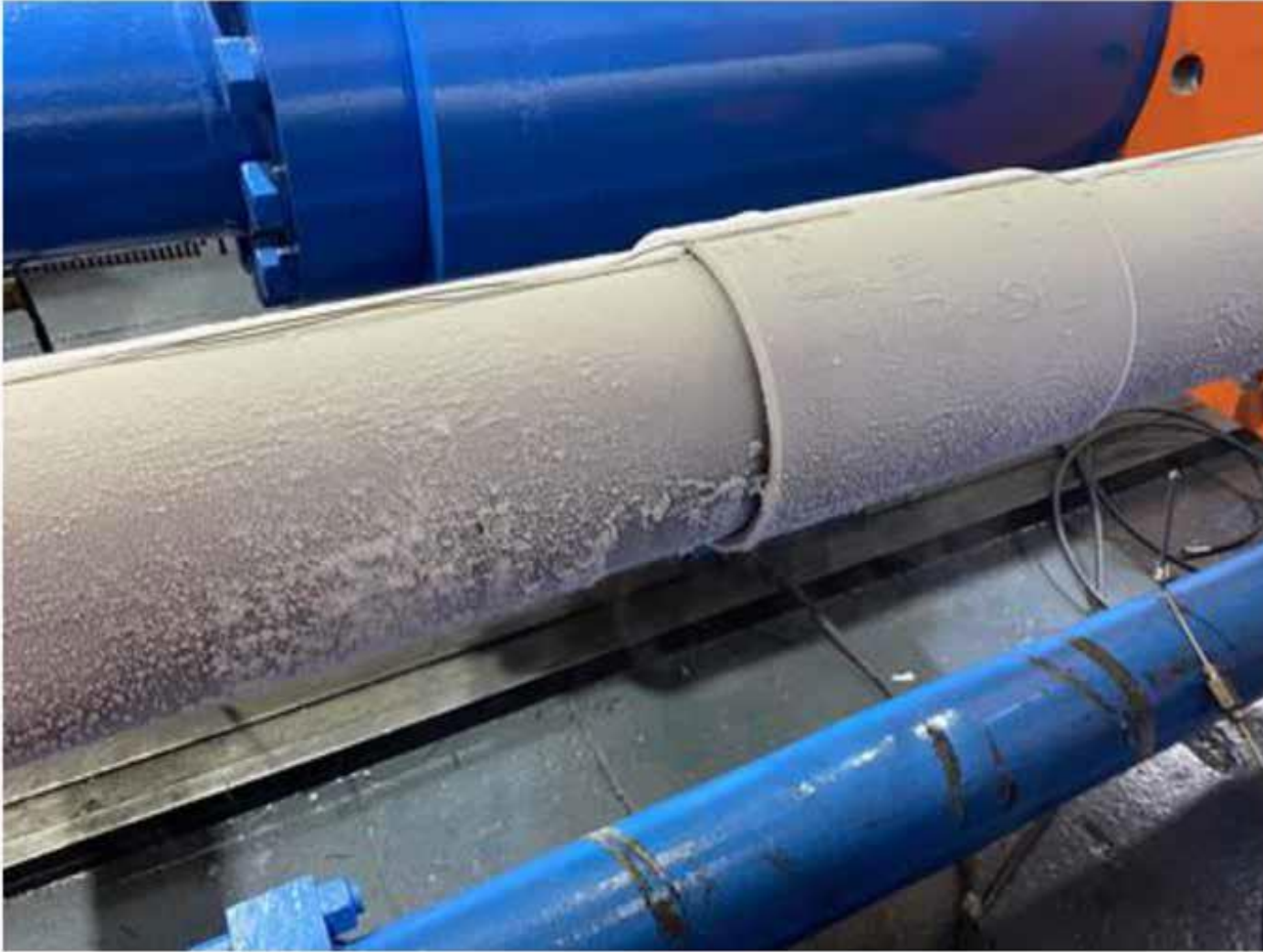
Specimen under testing after Thermal Shock test
