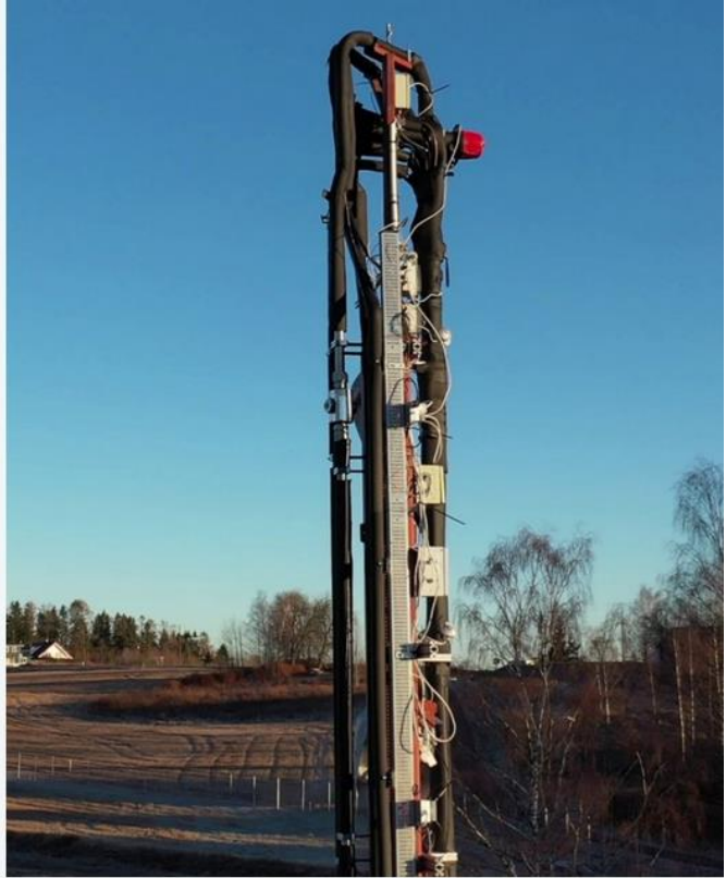
FALCON CO2 flow loop with the test section in vertical position.
