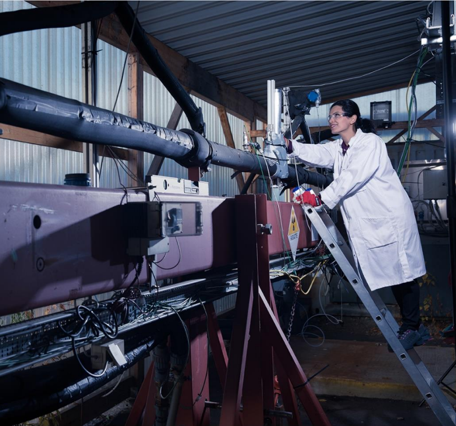
FALCON CO2 flow loop with an inclined test section. The inclination angle can be changed from full horizontal to full vertical
