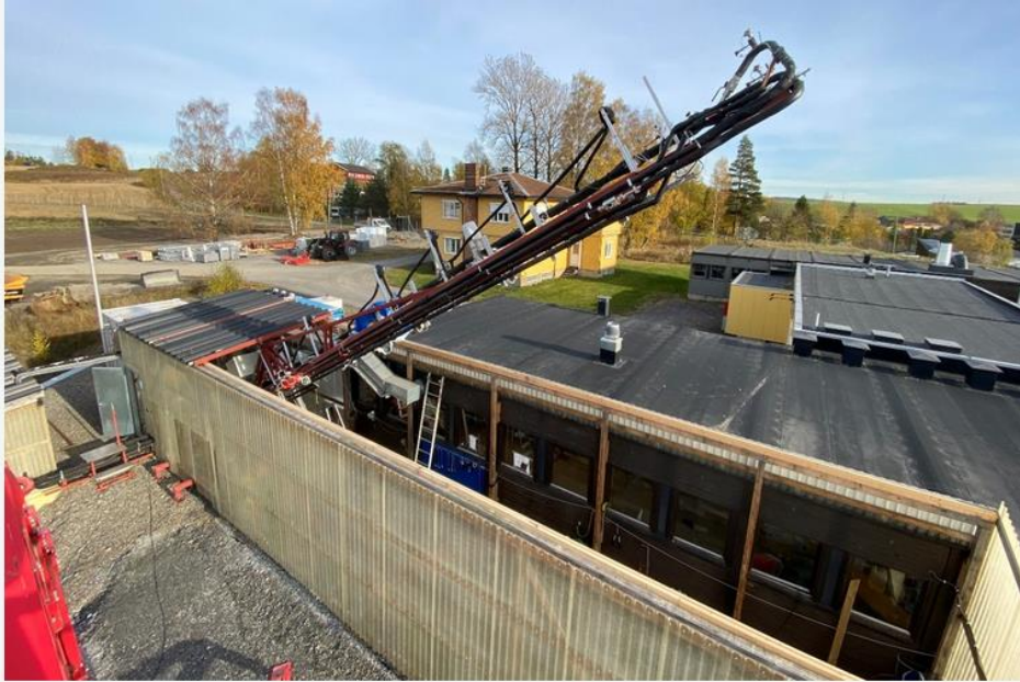
FALCON CO2 flow loop with an inclined test section. The inclination angle can be changed from full horizontal to full vertical
