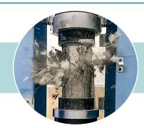
Test protocol mainly based on comparing performance and chemical-physical characteristics of the cement, before and after CO<sub>2</sub> exposure under the pressure and temperature conditions of the storage
