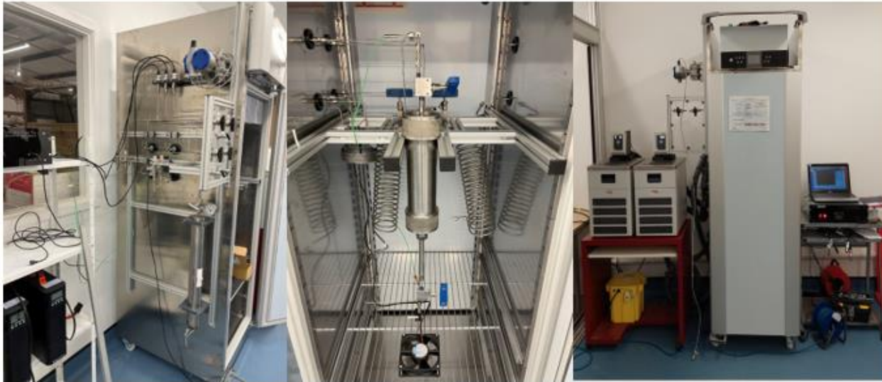
Figure 1: Dynamic Low Temperature CO 2 Injection Rig: Side View; Inside View; Front View with Door Closed (from left to right).
