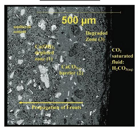
Kutchko et al., 2008. Rate of CO<sub>2</sub> attack on hydrated class H well cement under geologic sequestration conditions
