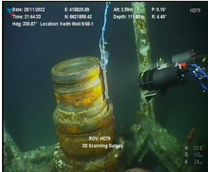
Wellhead surveillance/Subsea laser scanning (Savante)
