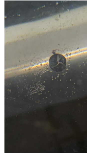
Successfully penetrating Inconel 718 with 10mm millbit
