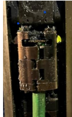
Gripper locked onto control line
