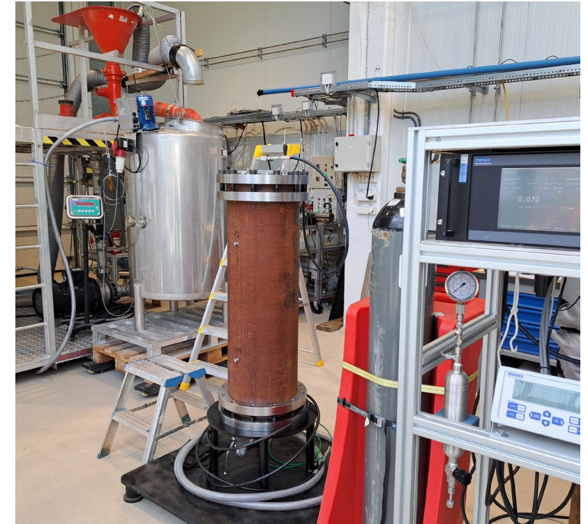
Annular cement integrity before, during and after setting a Bismuth alloy plug
