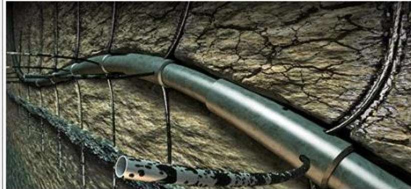
This technology involves drilling of «fishbones» into the reservoir from the main well.
