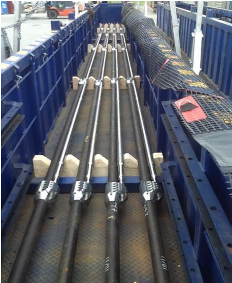
Example of Wireless Gauges Clamped to tubing and Wireless Subsea Receiver installed onto the debris cap
