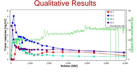
The dynamic model was updated with the detailed completion well design and production history, matching the well sections contribution with RESMAN results, **successfully forecasting water breakthrough**
