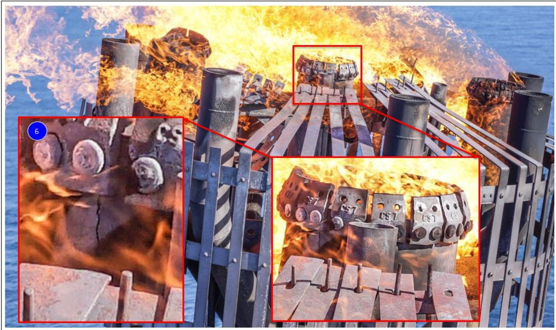
Small crack-like-indication found on HP upper shell, adjacent to the flame retention segments. Propagation likely under normal operating conditions and shutdown/start up (cooling).
