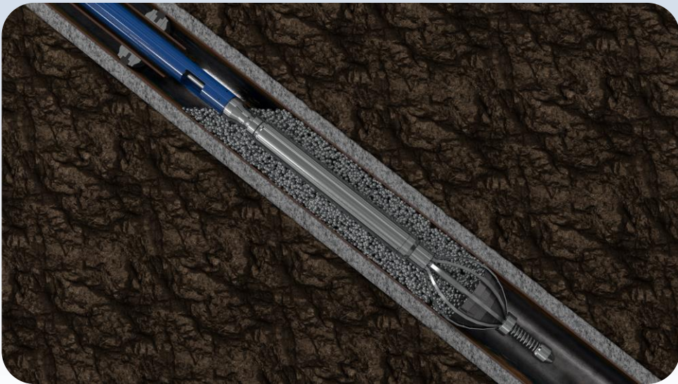
Alloy beads deployed in a bailer
