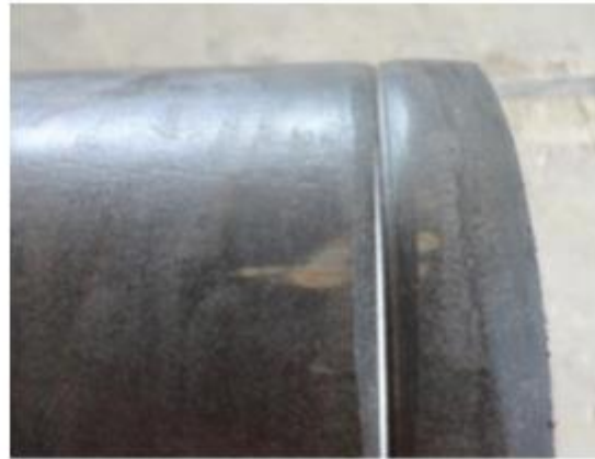
Photo 5: Pin end – Groove quality check
