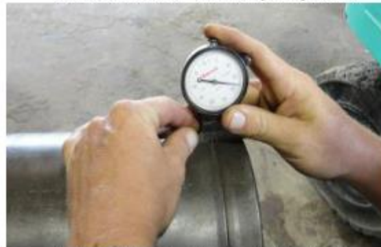
Photo 7: Pin end – Groove depth check
