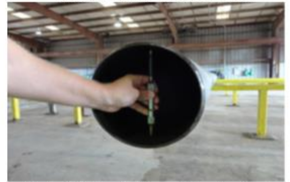
Photo 8: Bell end – Internal Diameter check
