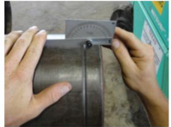
Photo 6: Pin end – turndown check
