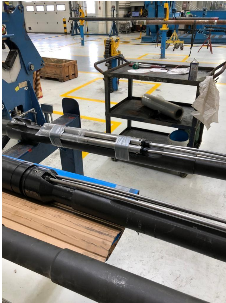
Two subassemblies splices above packer in back
