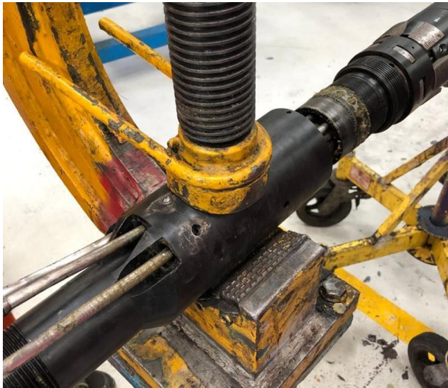
Packer top sub installation
