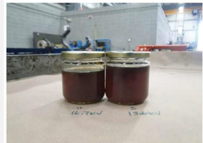
Oil samples collected from the motor: Head = 16.7 kV, Base = 13.6 kV
