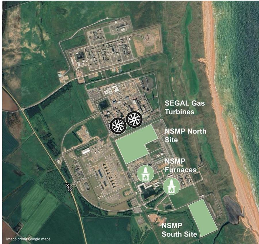
The current leading concept is that the carbon capture plant will be located at the NSMP North site and the Compression and Conditioning plant will be located on NSMP South site
