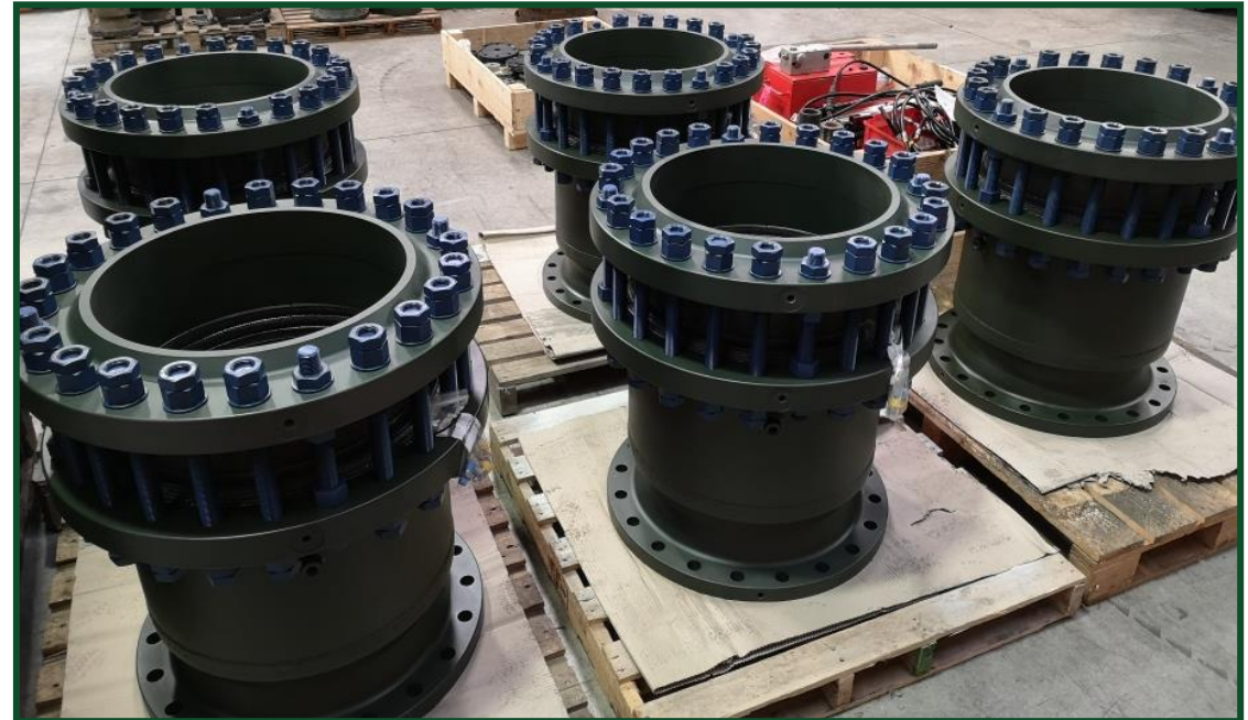
5 x 20" Connectors for a Flare System Replacement
