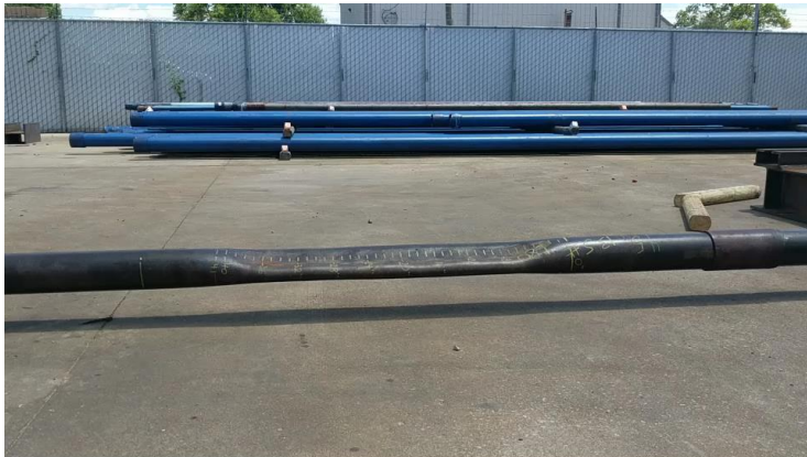
Crushed Pipe Prior to full scale test
