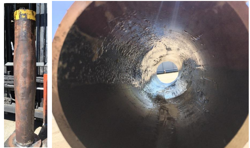
4.760" OD Cone 2 nd Pass – Before and After
