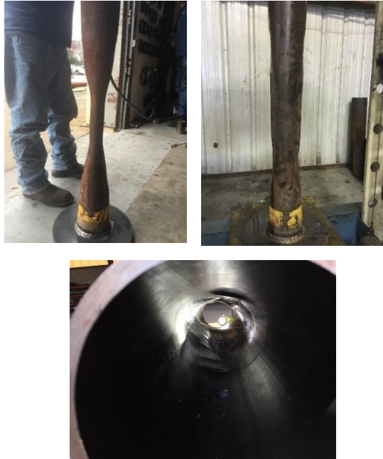
3.250" OD Cone Pass – Before and After
