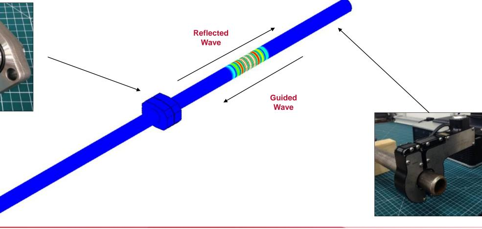
Using Ultrasonic Guided Wave NDT to investigate the feasibility of remotely inspecting pressure retaining O-rings in bolted connections
