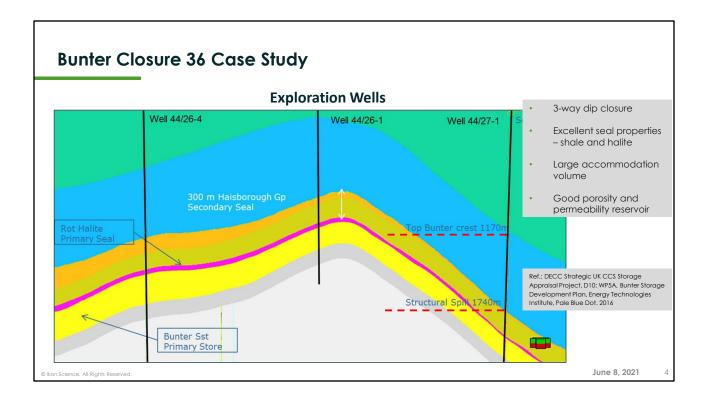
On this slide is shown a cross section through the Bunter reservoir.
