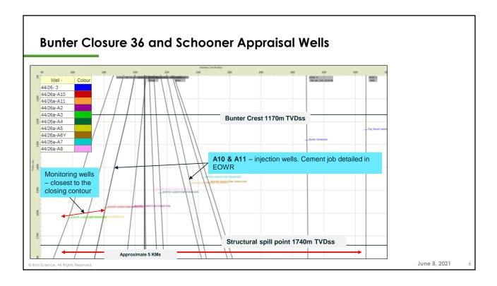
These two wells are shown in the cross section and given their position in the structure A10 is closer to the spill point and may be better suited as a CO2 monitoring well whereas A11, nearer to the crest, is better placed as an injector.
