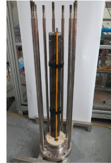
Figure 16: Modified 8 inch dual casing set-up (open)
