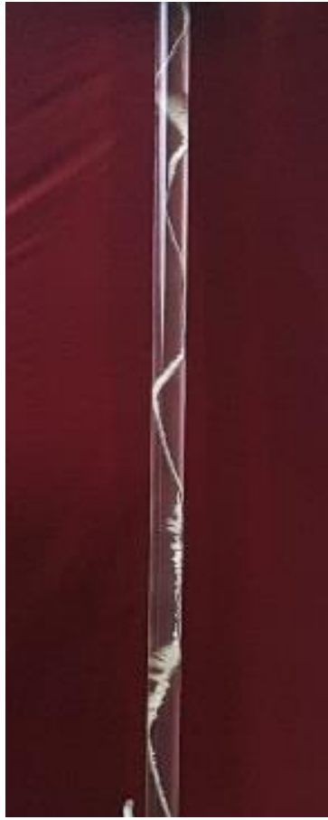
Extent of scaling after 24 hours.
