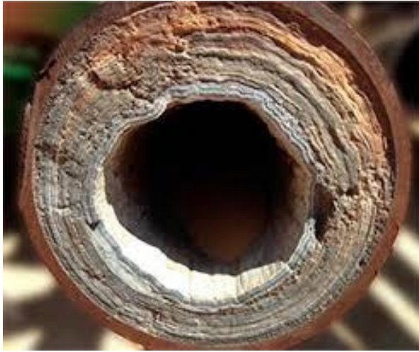
Pipeline contaminated with inorganic scale (Mady and Kelland, 2020).
