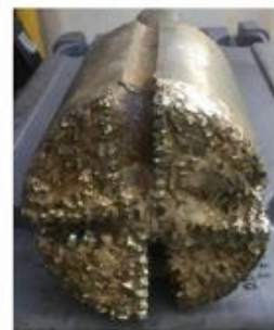
After underreamer run – expected wear
