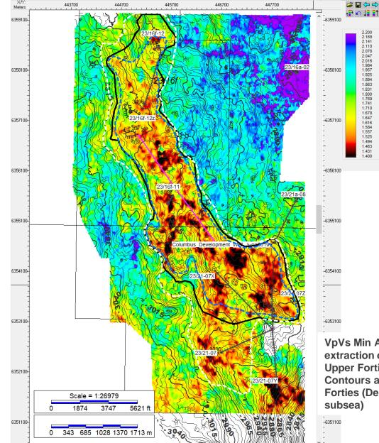
VpVs Min Amp. extraction over the **Upper Forties Inteval; Contours at Top** Forties (Depth,
