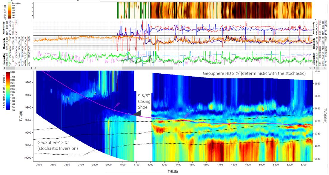
• GeoSphere used to verify correct structural setting vs. Forties Sands (warmer colours) below well path on final approach.
