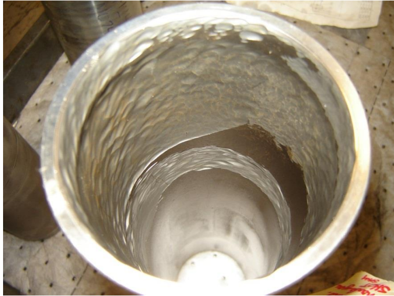
Gas Separator Compression tube @ 25 hrs. Abrasive Loop Testing
