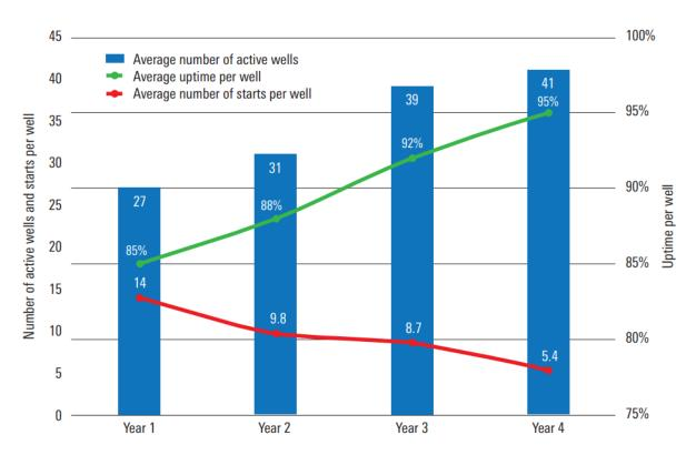
Lift IQ service increased ESP uptime to 95% while reducing the number of starts per well per year from 14 to 5.4, thereby improving system survivability.
