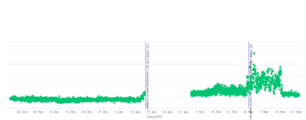
Fig 2. Sudden increase spectral energy at rotational frequency of the motor
