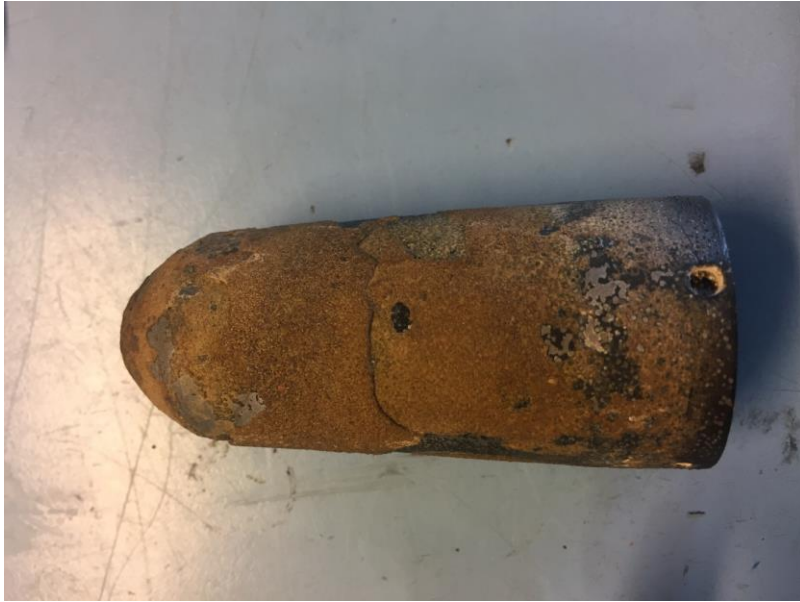
Scale formation on the outer part of the valve
